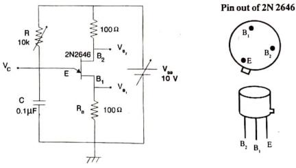
**Design Output requirements** Amplitude and frequency of sweep waveform = 10 V, 1 kHz. **DC bias conditions**  $V_{cc} = 10$  V since the required amplitude of the output = 10 V
