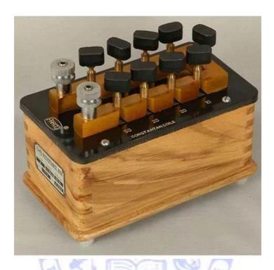
A resistance box, also known as a decade box or resistance substitution box, is a specialized electrical device used to provide precise and variable electrical resistance in electronic and electrical circuits. Here's an explanation of its key features and uses:
