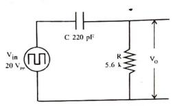
Let the input be a pulse train of 1 kHz. Then T = 1 ms. Design
