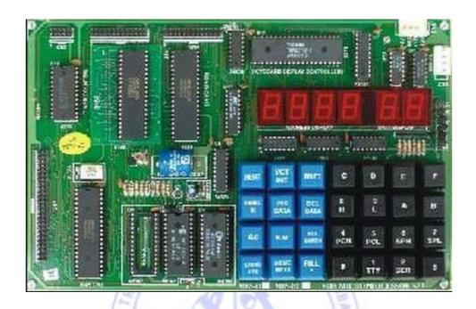
The Intel 8085 is a microprocessor that was widely used in the late 1970s and early 1980s. Here are some key points:
