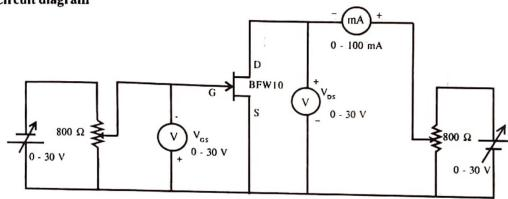
Details of BFW 10/11 Type N-channel JFET,  $I_d = 2mA$ ,  $g_m = 2.5 \text{ mA/V}$ ,  $R_O = 40 \text{ k}$
