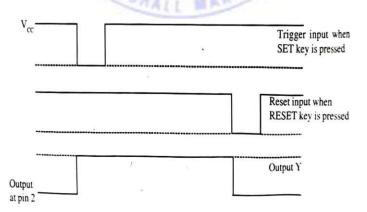
Similarly when switch RESET is pressed, the output at pin 3 becomes LOW.
