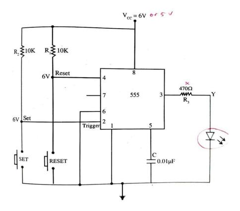
SET and RESET are controlled by two switches. LED is working as an output indicator. When the above two switches are open, second and fourth pins will be HIGH. When these switches are closed, they become LOW. C is used for eliminating high frequency noises. The resistor R, is used for limiting the current through LED.
