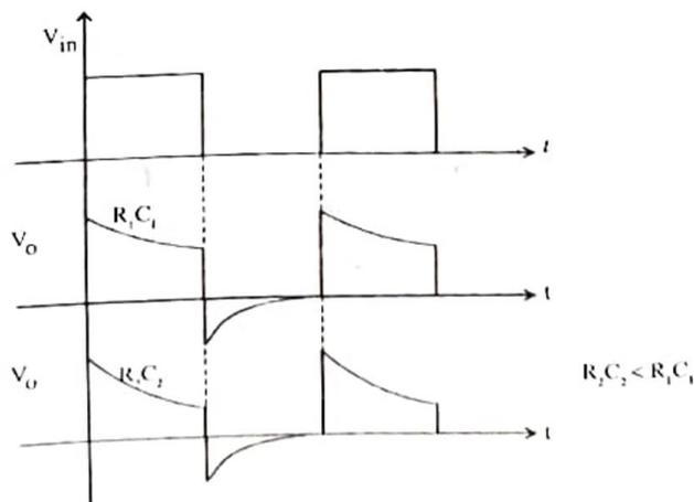
Response of the RC differentiator to a pulse train input
