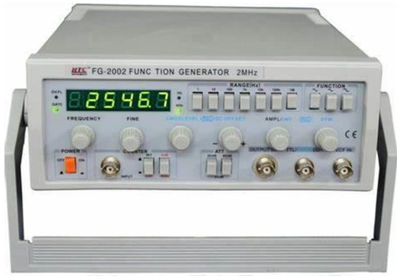
A function generator is a type of electronic test equipment used in various fields, including electronics, engineering, and physics. It is designed to produce precise and controllable electrical waveforms, such as sine waves, square waves, triangular waves, and more. Here are some key points about function generators:
